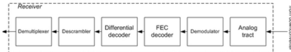
Fig 9. DVB-S receiver block diagram.
