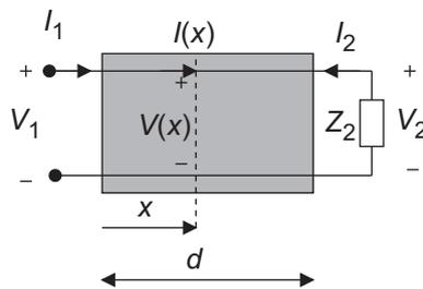
Figure 1: Loaded transmission line.
